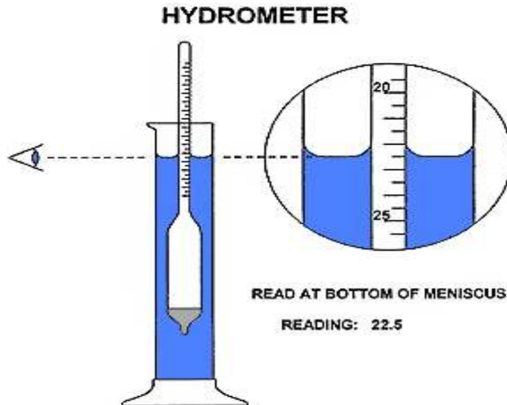
**Figure 2 - Operation of the hydrometer is based on the principle that a solid suspended in a fluid will be buoyed up by a force equal to the weight of the fluid displaced by the submerged part of the suspended solid. Thus, the lower the density of the substance, the farther the hydrometer will sink.**
